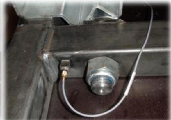
The last accelerometer was installed onto the central beam in a radial direction and should examine the magnitude of the dynamic effects acting during the drive.
